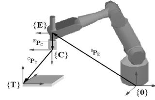
Figure 3. Frame assignment for vision-based control.
