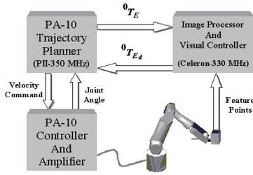
Figure 5. Hardware configuration for vision-based control system.
