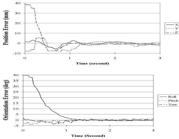
Figure 9. Relative target pose error when using PI control in visual control loop: inaccurate eye-hand relationship.
