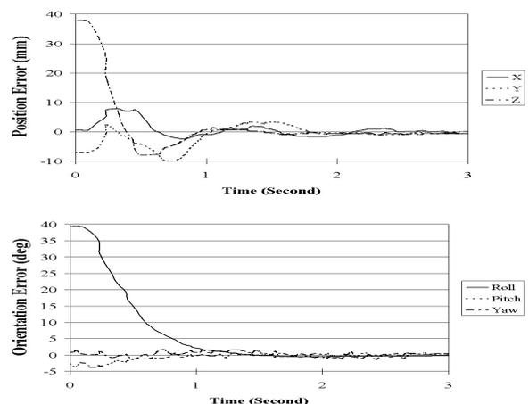
Figure 8. Relative target pose error when using PI control in visual control loop: accurate eye-hand relationship.
