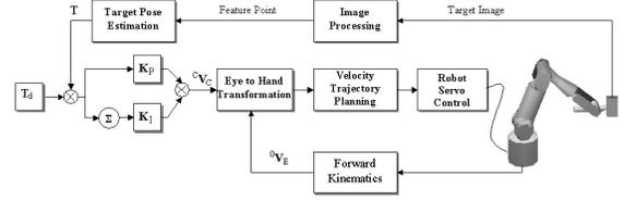
Figure 4. Visual control system structure.
