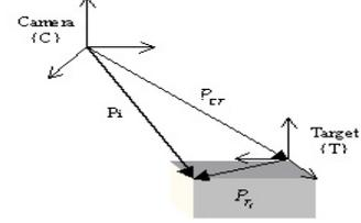
Figure 2. Target and camera coordinate frame.
