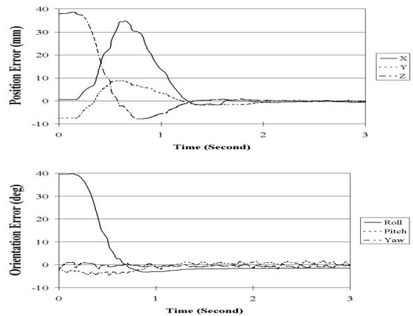
Figure 6. Relative target pose error when using kinematics calculation: accurate eye-hand relationship.
