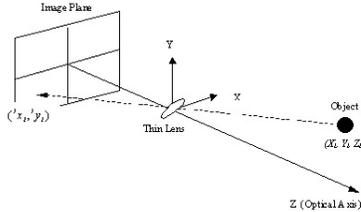
Figure 1. Pinhole camera model.
