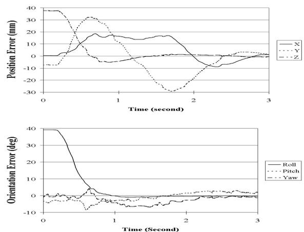
Figure 7. Relative target pose error when using kinematics calculation: inaccurate eye-hand relationship.
