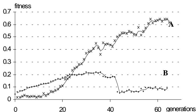
Figure 8: The curve A illustrates the successful development of the wall following behavior when the initial population used is from end of stage I, while curve B illustrates that incremental evolution did not succeed when the initial population was from end of stage II.
