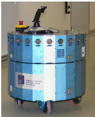
Fig. 1. Omnidirectional mobile robot with 4 powered caster wheels.
