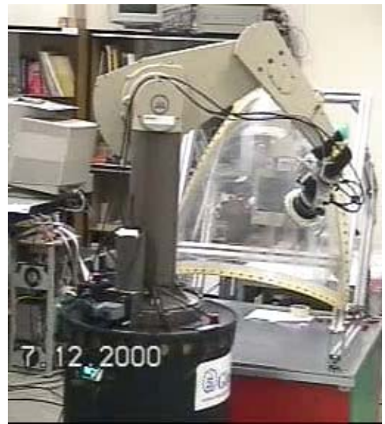
Figure 1: Mobile manipulator setup polishing an aircraft canopy
