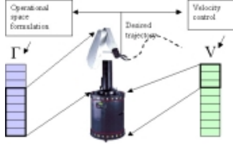
Figure 1. Torque vector from operational space formulation and velocity vector from velocity control, are both generated to satisfy the desired trajectory. The commands are sent to the corresponding joints.
