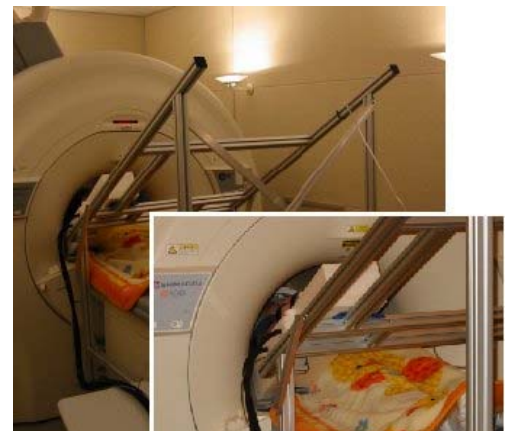
A fMRI compatible haptic interface with hydrostatic transmission installed at ATR
