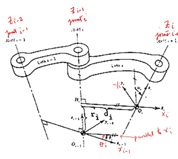
Rotate an angle of  $\theta i$  (in the right-handed sense) about the zi-1 axis, so that the xi-1 axis is parallel to the xi axis.
