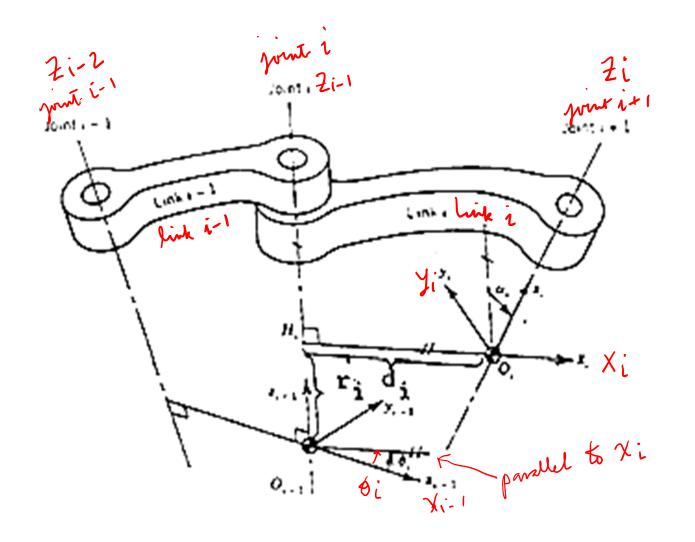
the  $z_i$  axis is directed along the axis of motion of joint (i + 1), that is, link (i + 1) rotates about or translates along  $z_i$ ;
