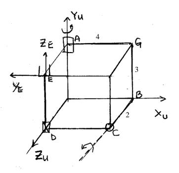
1<sup>st</sup> link: AGBC (rotating) 2<sup>nd</sup> link: CD (rotating) 3<sup>rd</sup> link: ED (translating)
